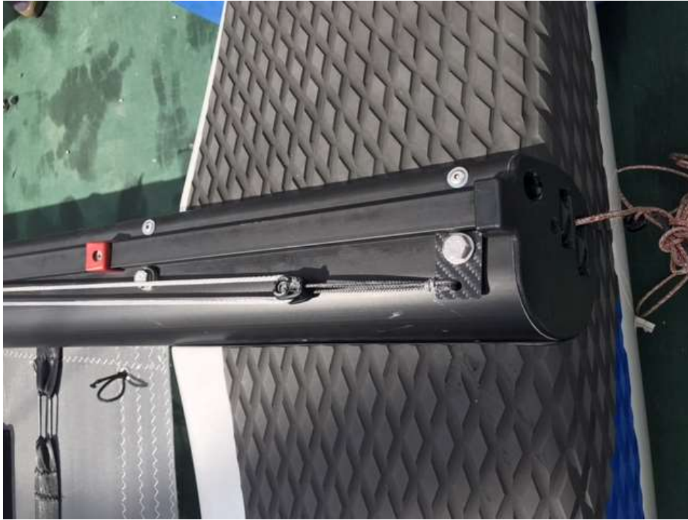
Figure 1 - Bullet block addition off aft crossbar bolt
